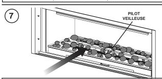
RANDOMLY PLACE THE ROCKS ONTO THE MEDIA TRAY, AROUND, BUT NOT ON THE BURNER PORTS OR PILOT AREA. PLACER LES ROCHES SUR LE PLATEAU, AU TOURS, MAIS PAS SUR LES PORTS DE BRÛLEUR OU VEILLEUSE.
